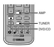
As shown on the left, CinemaStation is composed of three main parts. Remote Control button operations change depending on the mode, so it is possible to control all Amplifier, DVD/CD and Tuner functions with a single remote unit.
