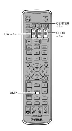
Adjust the volume level of the Subwoofer, Center and Surround Left/Right Speakers, if you feel the speaker is unbalanced during audio playback.
