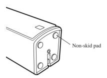
As shown in the picture, attach the non-skid pads on the bottoms of the Front and Surround Speakers in the four corners. This stabilizes the speakers to prevent sliding.
