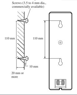
Attach to the wall using the two holes on the back of the Front and Surround Speakers.
