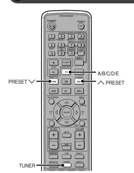
You can tune in a radio station simply by selecting its Preset Number.
