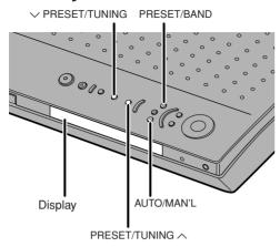
For stations with weak radio signals, tune manually.
