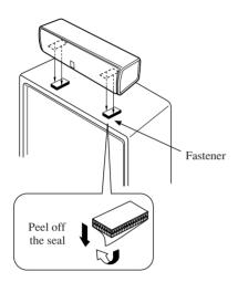
Make sure the top of the television is level. If the top of the television is not level, place the Center Speaker inside the TV rack or directly on the floor. In any case, make sure it is placed on a level surface.
