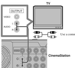
Enjoy TV sound with CinemaStation by connecting the TV audio output jack to the audio IN jacks of VIDEO 1 or VIDEO 2 ("VIDEO" IN jack on U.K. and Europe models). Press VIDEO 1 or VIDEO 2 on the Remote Control to input TV sound.
